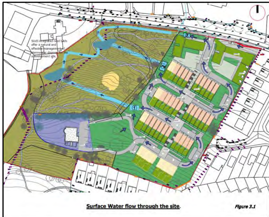
Figure 17: Potential Surface Water Drainage Design
